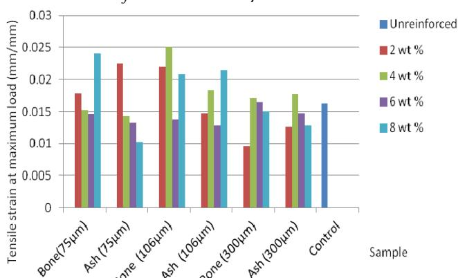
Figure 3. Variation of Tensile Strain at Maximum Load with Particle Sizes for both Cow Bone and Cow Bone Ash Reinforced Composites
