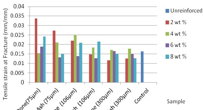
Figure 5. Variation of Tensile Strain at Fracture with Particle Sizes for both Cow Bone and Cow Bone Ash Reinforced Composites
