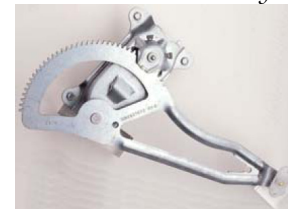
Figure 3. Single arm driver mechanism
