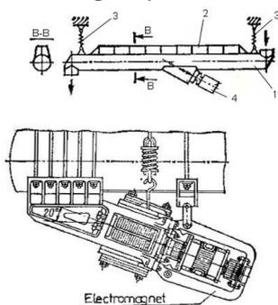
Figure 2. Vibrating sieve electromagnetically driven
