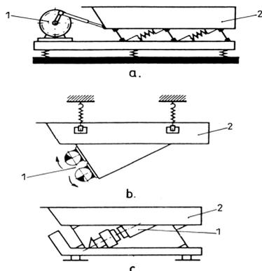
Figure 1. Basic types of vibrating feeders:
