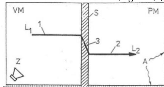
Figure 1. The principle of definition airborne sound insulation of the building construction
