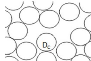
Figure 1A: Kozeny-Carman's model of porous sheets
