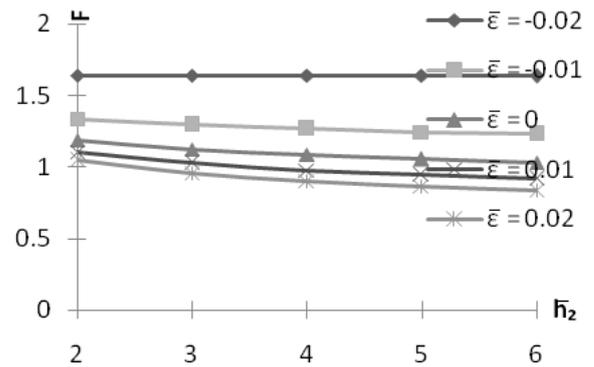
Figure 18: Variation of Friction with respect to  $\bar{h}_2$  and  $\bar{\epsilon}$ .
