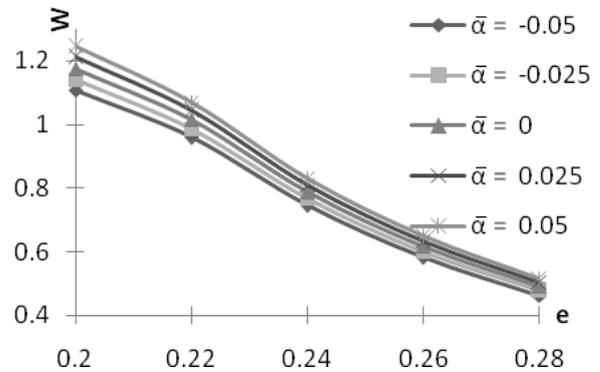
Figure 12: Variation of load carrying capacity with respect to  $e$  and  $\bar{\alpha}$ .
