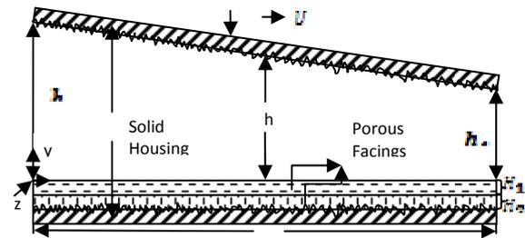
Figure 1: Configuration of the bearing system
