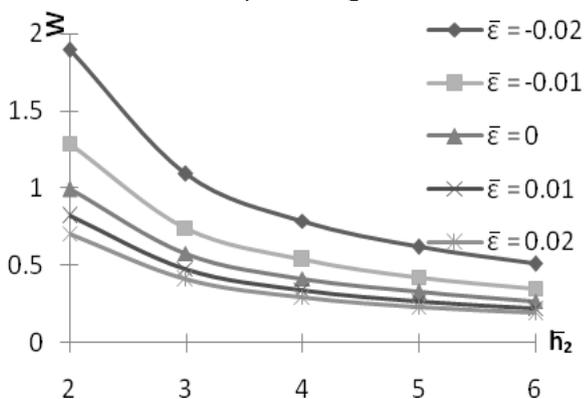
Figure 4: Variation of load carrying capacity with respect to  $\bar{h}_2$  and  $\bar{\epsilon}$ .
