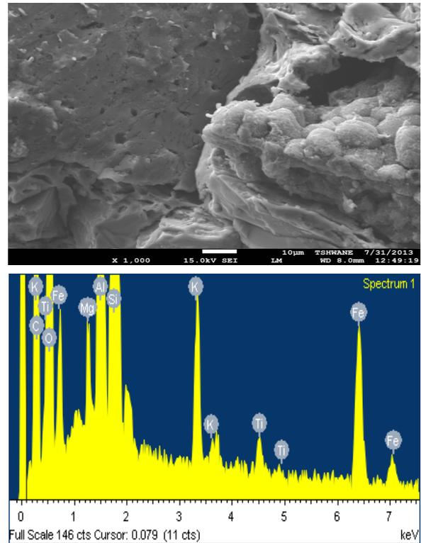
Figure 9: SEM/EDS Microstructure of the 50 % carbonized palm kernel shell addition
