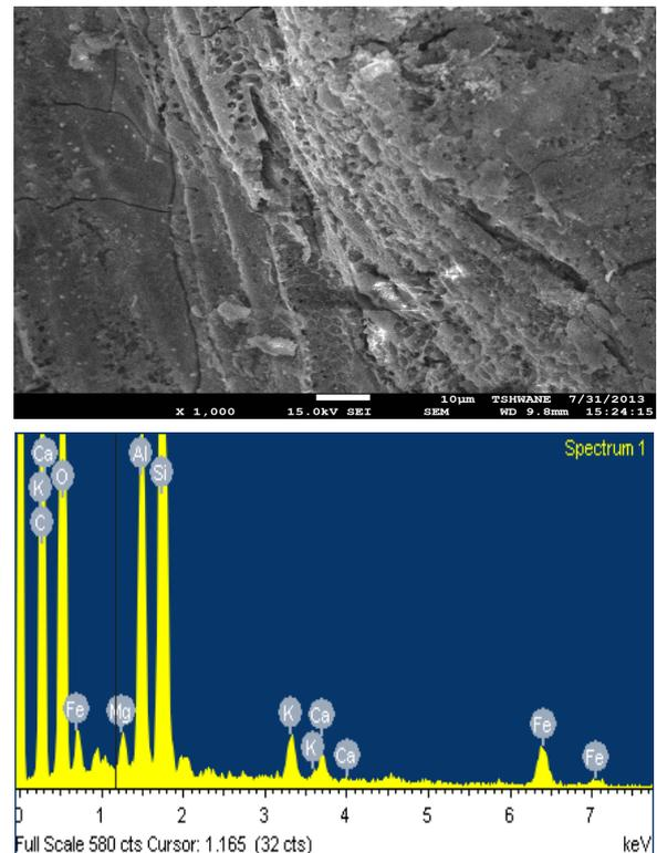
Figure 10: SEM/EDX Microstructure of the 60 % carbonized palm kernel shell addition
