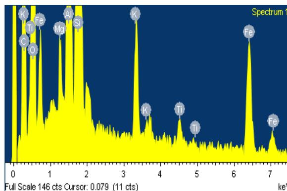
Figure 9: SEM/EDS Microstructure of the 50 % carbonized palm kernel shell addition
