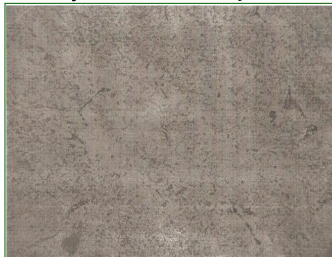
Figure 2. Microstructure of Die Casting (X400)
