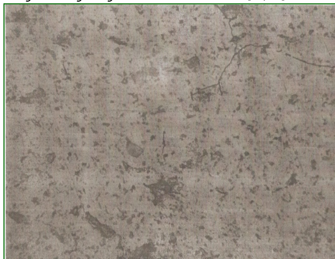
Figure 1. Microstructure of Sand Casting (X400)
