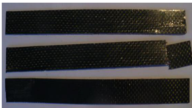
Figure 6: Beaked samples after testing (samples JV1, JV2, JV3)
