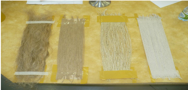
Figure 2: 2 nd type of natural fibres sample made from straight laid 25cm fibres
