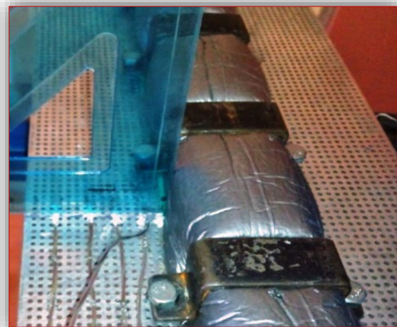
Figure 4. Thermocouples positions on the perforated plate
