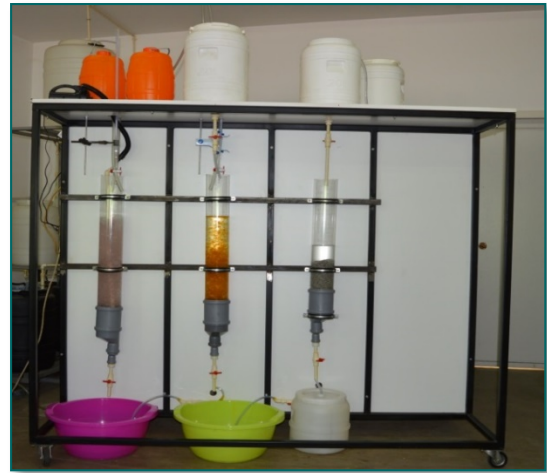
Figure 2. Pilot plant for the treatment of raw drinking water by ferrate(VI) ferrate(VI)
