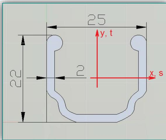
**Figure 1.** Cross section of the rim
