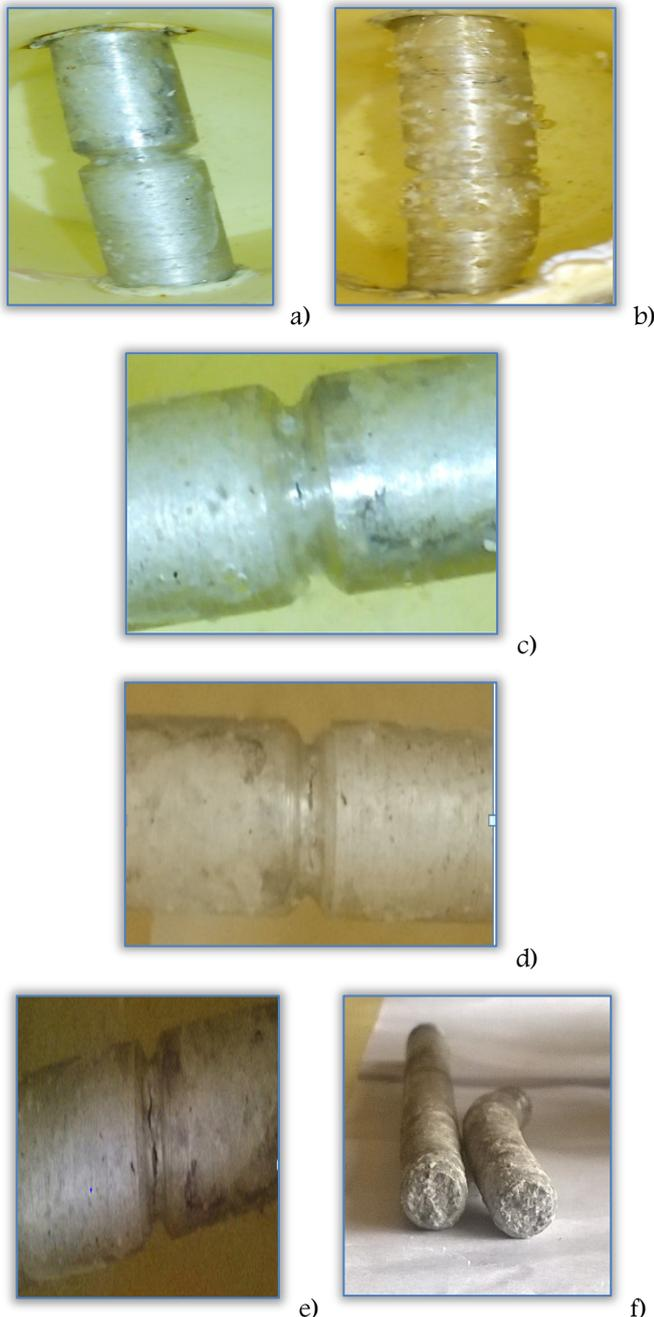
Figure 4: Representative photomicrographs showing the nature of macroscopic crack evolution to final fracture in the test specimen (a) after 4 days of testing, (b) for 9 days of testing, (c) 15 days of testing, (d) 25 days of testing, (e) 35 days of testing, (f) fracture on 40<sup>th</sup> day of testing
