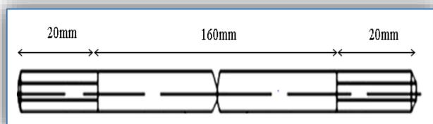
Figure 2: Specimen specification for circumferentially notched cylindrical bar samples
