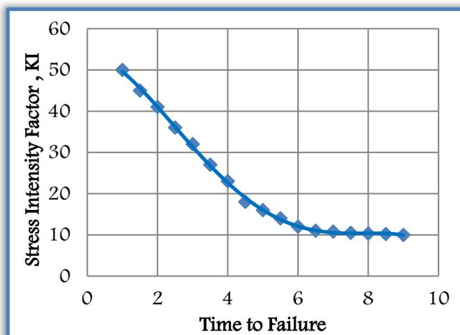
Figure 3: A schematic plot of stress intensity against time to failure (tff)
