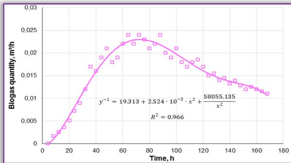
Fig. 4 - Variation of biogas production at 45°C
