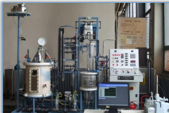
**Fig. 1 -** Small capacity plant for biogas production [8]
