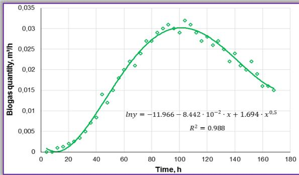
Fig. 3 - Variation of biogas production at 35°C
