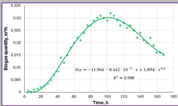
Fig. 3 - Variation of biogas production at 35°C
