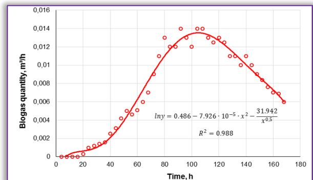
Fig. 2 –Variation of biogas production at 25°C
