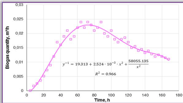
Fig. 4 - Variation of biogas production at 45°C
