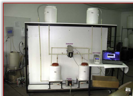
Figure 1. Device for electrochemical synthesis of ferrate (VI)
