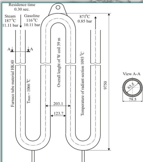
Figure 1. The radiant coil assembly
