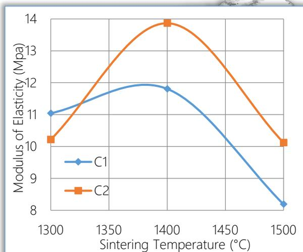
Figure 4. Effects of sintering temperature on the Young's modulus of elasticity of the samples
