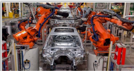
Figure 2 – Body shop - Best fit process [1]
