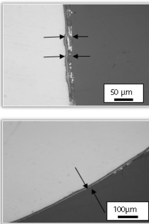
Figure 3a and 3b. Galvanized (zinc-coating) layer of the chains (thickness 16 mm)
