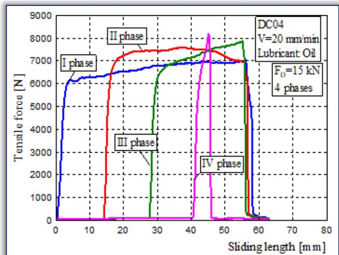
Figure 10. Tensile force vs. sliding length curves
