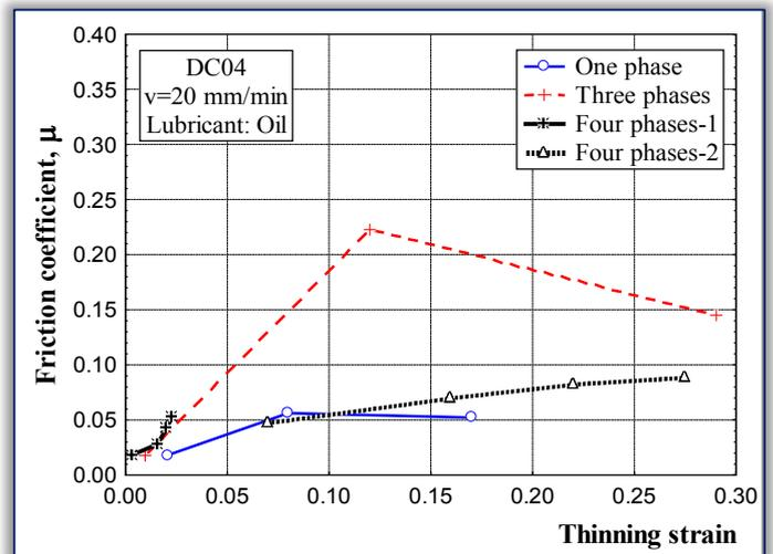
Figure 14. Friction coefficient dependence on thinning strain
