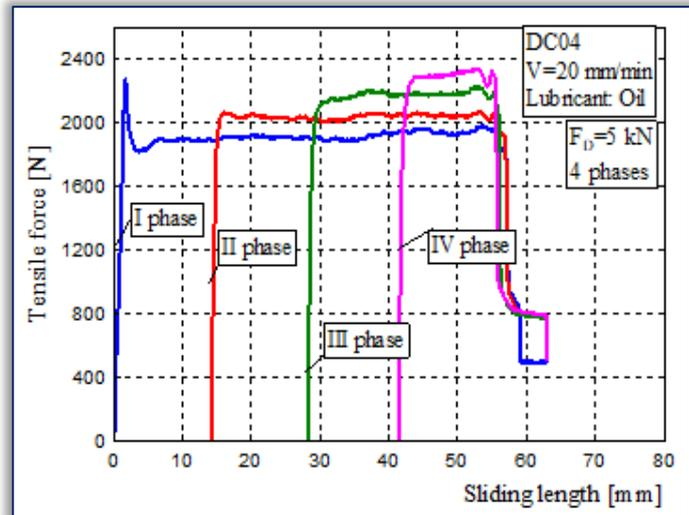
Figure 9. Tensile force vs. sliding length curves
