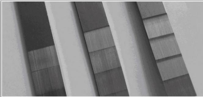
Figure 11. Strips after multi-phase ironing
