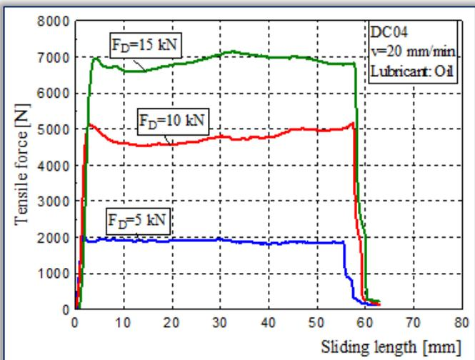
Figure 7. Tensile force vs. sliding length curves
