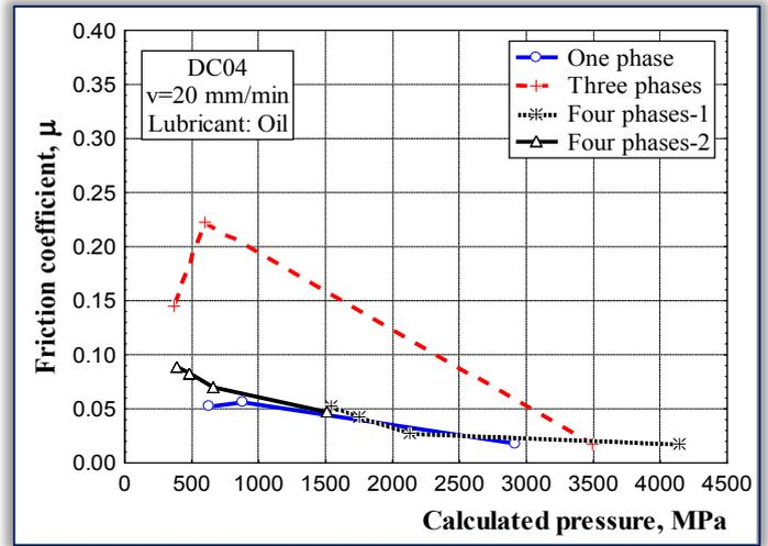
Figure 13. Friction coefficient dependence on calculated pressure
