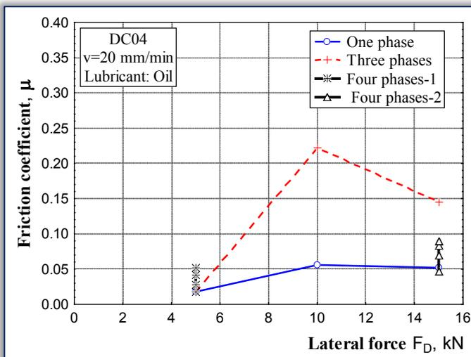
Figure 12. Friction coefficient dependence on lateral force
