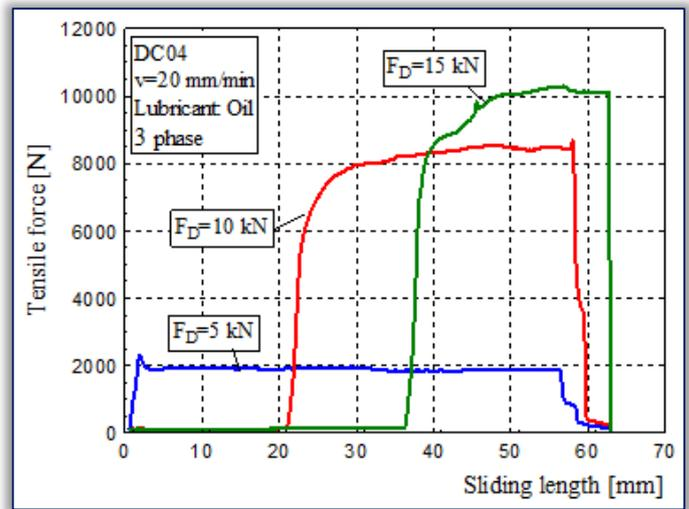
Figure 8. Tensile force vs. sliding length curves
