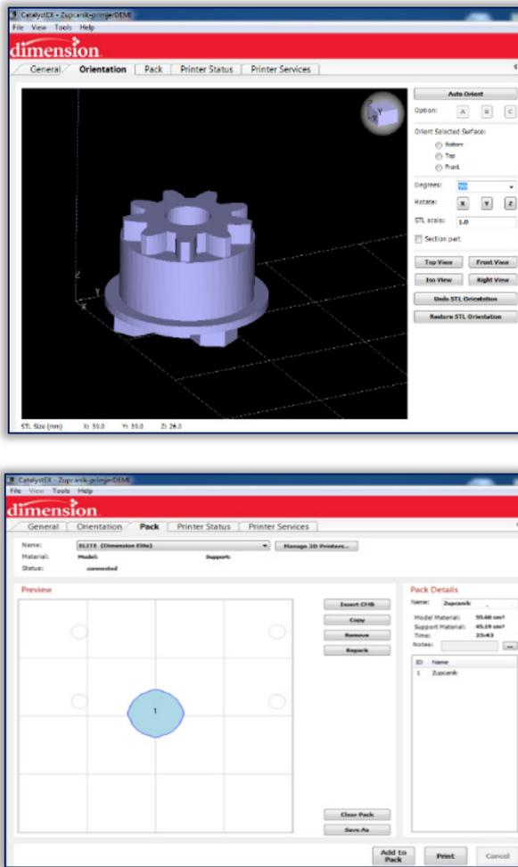
Figure 2. Orientation and processing of models in CatalystEX
