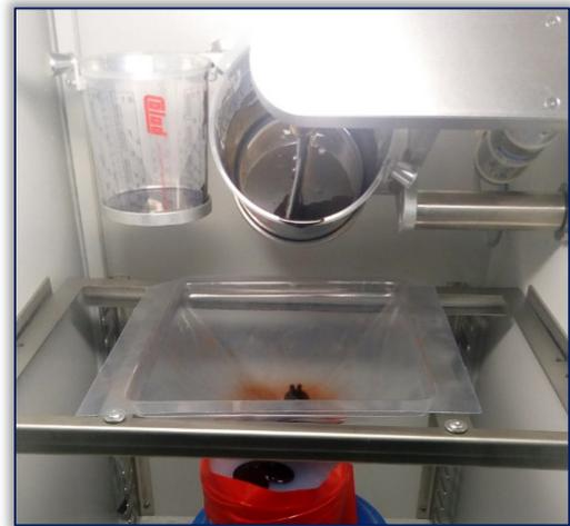
Figure 6. The casting process in a vacuum chamber MK-mini
