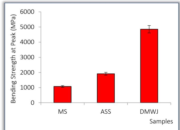
Figure 4: Bending Strengths of base metals and the dissimilar metal welded joint
