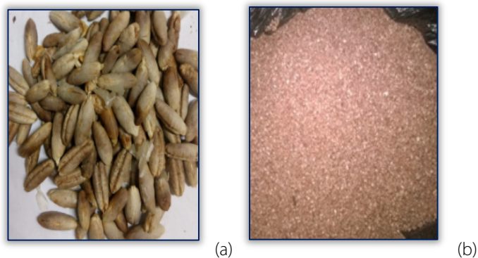
Figure 1. Date Seed Used in this Work (a) Raw Date Seeds and (b) Pulverized Date Seed
