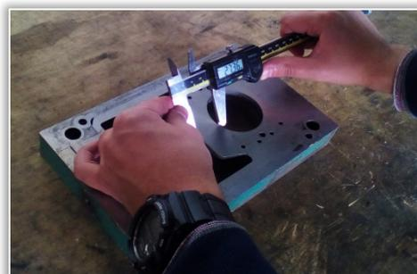
Figure 9. Measurement of tool part [8]
