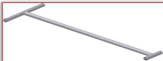
Figure 2. Pantograph mechanism connecting rod
