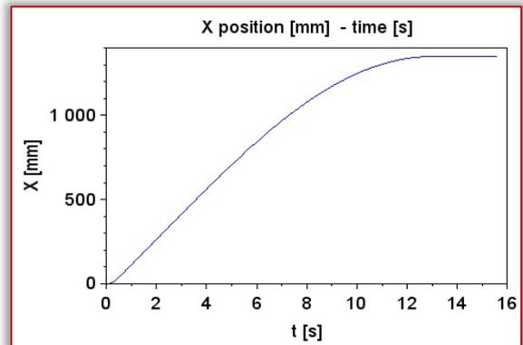
Figure 3. X position of the AGV during cornering
