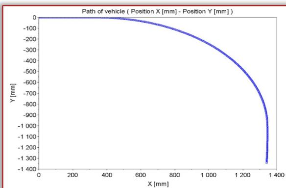
Figure 8. Path of the AGV during cornering
