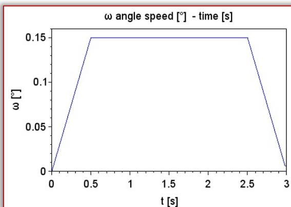
Figure 13. Angular velocity of the AGV during arch motion
