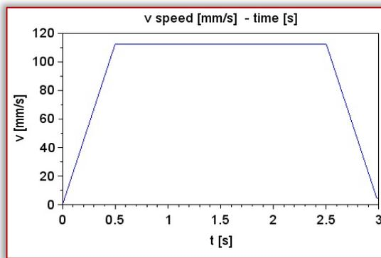
Figure 14. Velocity of the AGV during arch motion
