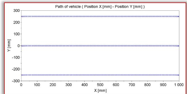
Figure 20. Path of the AGV during motion between two points
