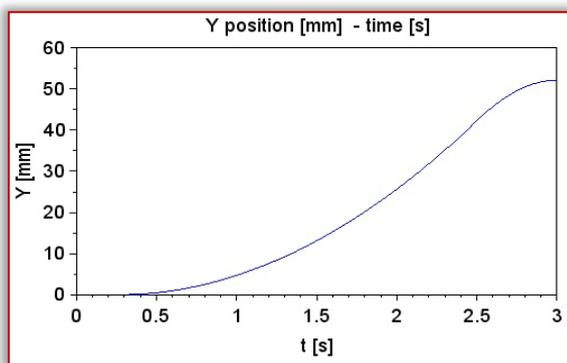
Figure 11. Y position of the AGV during arch motion
