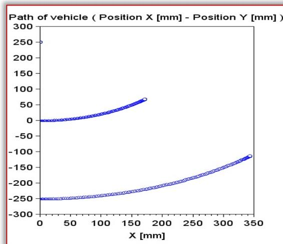
Figure 16. Path of the wheels and AGV during arch motion (only right wheel moves)
