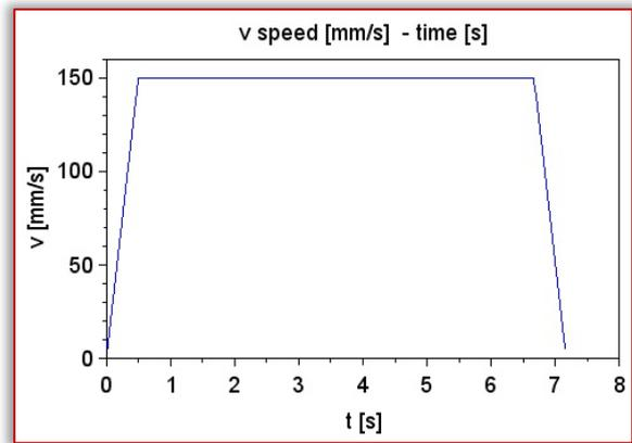
Figure 19. Velocity of the AGV during motion between two points
