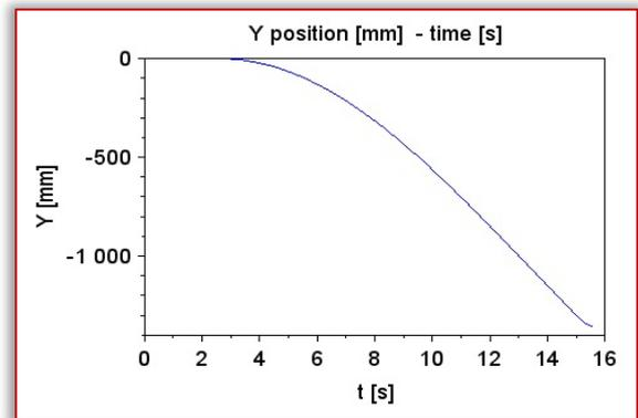
Figure 4. Y position of the AGV during cornering
