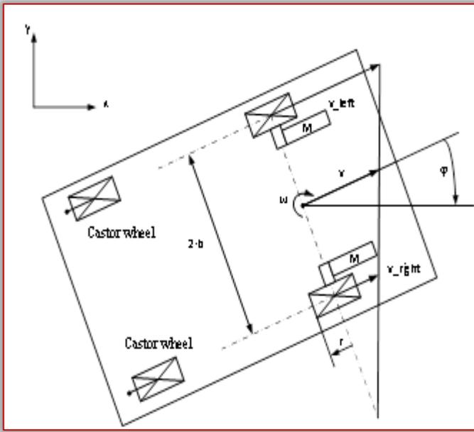
Figure 1. Kinematic model of the AGV
