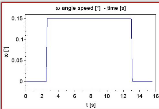
Figure 6. Angular velocity of the AGV during cornering
