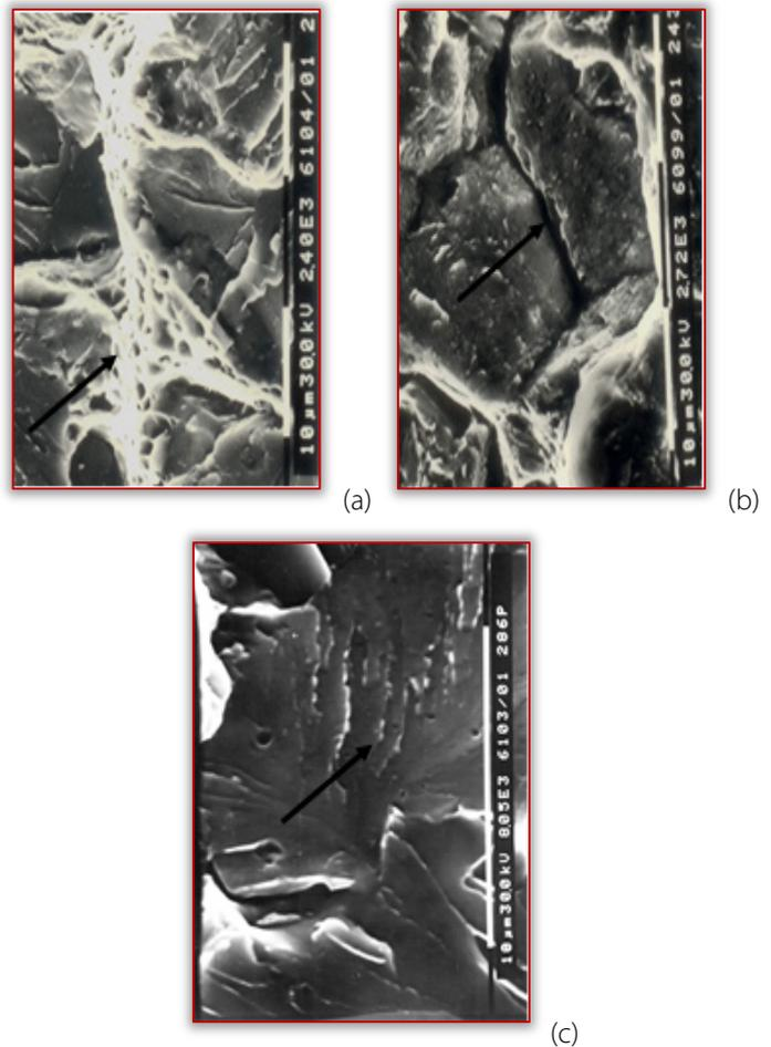
Figure 4 - Fractographs of thermally treated samples after annealing at: a, c - 600°C; b- 650°C
