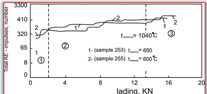
Figure 5 - Change of the total energy with respect to the load of the studied samples
