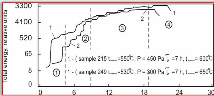
Figure 8 - Total energy change with respect to the load for the nitrided samples
