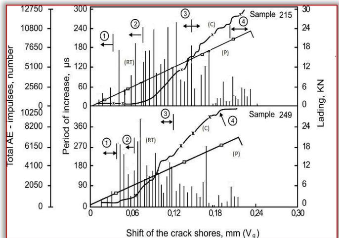
Figure 7 - Change of the AE-parameters and the load with respect to the displacement of the crack banks for the ion-nitrided samples 215 and 249
