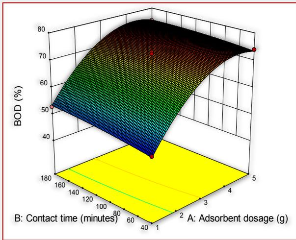
Figure 1: Response surface plot showing predicted BOD reduction as a function of adsorbent dosage and contact time with temperature fixed at 35°C.
