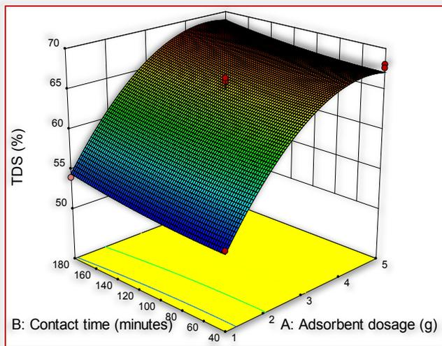
Figure 7: Response surface plot showing predicted TDS reduction as a function of adsorbent dosage and contact time with temperature fixed at 35°C.
