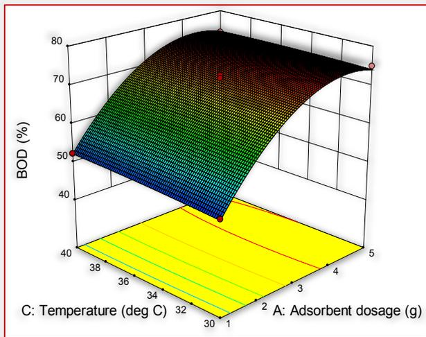
Figure 2: Response surface plot showing predicted BOD reduction as a function of adsorbent dosage and temperature with contact time fixed at 110minutes.
