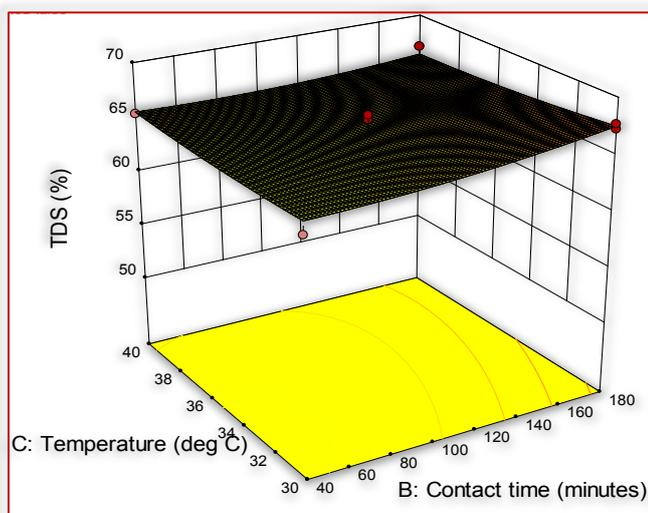
Figure 9: Response surface plot showing predicted TDS reduction as a function of contact time and temperature with adsorbent dosage fixed at 3g
