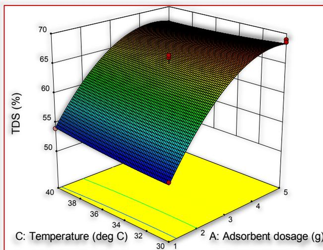
Figure 8: Response surface plot showing predicted TDS reduction as a function of adsorbent dosage and temperature with contact time fixed at 110 minutes
