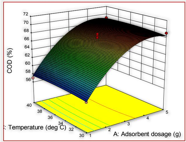
Figure 5: Response surface plot showing predicted COD reduction as a function of adsorbent dosage and temperature with contact time fixed at 110minutes.
