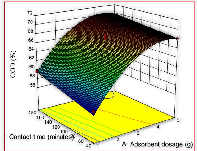
Figure 4: Response surface plot showing predicted COD reduction as a function of adsorbent dosage and contact time with temperature fixed at 35°C.
