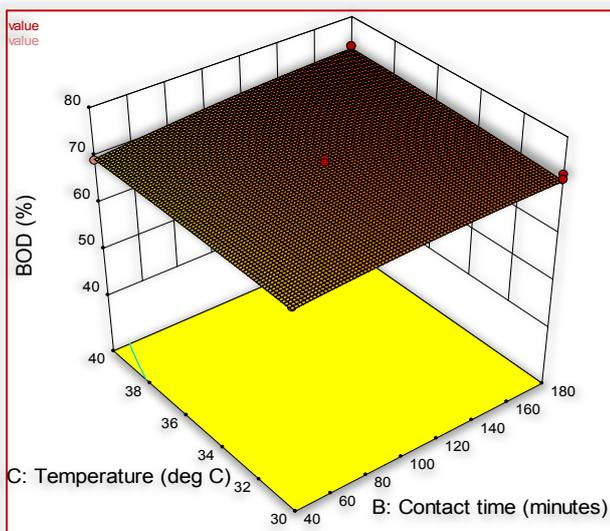
Figure 3: Response surface plot showing predicted BOD reduction as a function of contact time and temperature with fixed adsorbent dosage at 3g.
