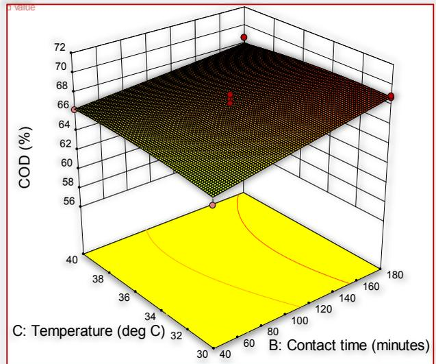
Figure 6: Response surface plot showing predicted COD reduction as a function of temperature and contact time with adsorbent dosage fixed at 3g.
