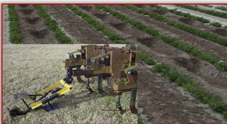
Figure 6 - Open furrow machine compartmented over a single interval [9]
