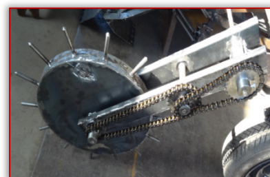
Figure 9 - Chain transmission for driving the rotor control mechanism [6]
