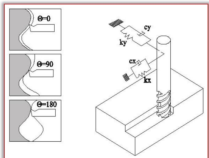
**Figure 1.** Regenerative chatter in milling. Initial tool deflection copied to workpiece surface is encountered in the next tool revolution
