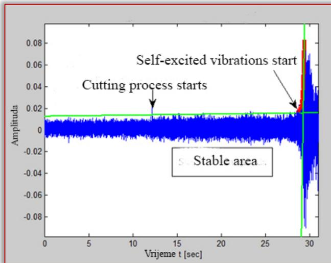
Figure 3. The amplitude of vibration in time domain and occurrence of self-excited vibration
