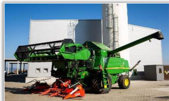
Figure 5 – Combine of harvesting hemp seeds, stems and leaves [2,3] HempFlax, a Dutch company established since 1994, is designing, developing and patenting equipment specialized in hemp cultivation, offering an innovating combine able to perform three different harvesting operations at the same time, namely hemp seeds, stems and leaves harvesting. [2,3]
