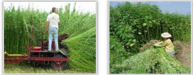
Figure 4 – Hemp harvesting machine, [14]
