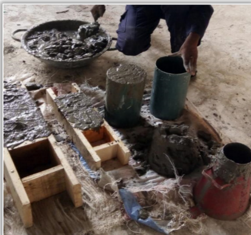
Figure 3. Concrete workability test using slump cone
