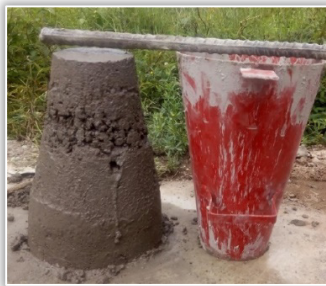
Figure 3. Concrete workability test using slump cone
