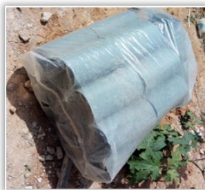
Figure 4: Concrete moulds for Compressive Strength and Tensile Strength tests
