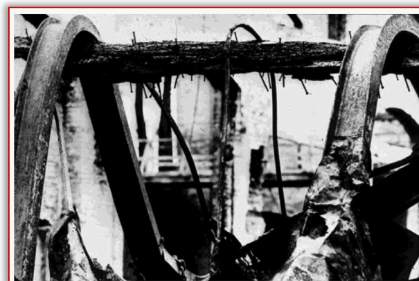
Plate 2. Wood beam survives fire in casein plant Frankfort, NY. Courtesy; Handbook of Wood Chemistry and Wood Composites Second Edition, 2013
