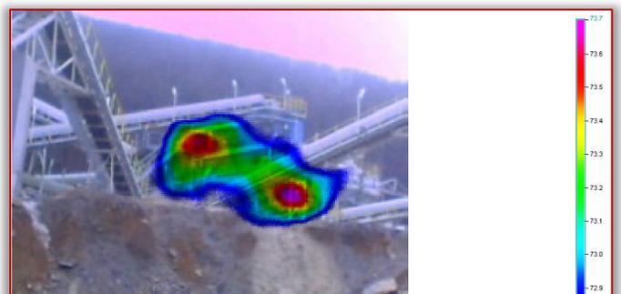
Figure 8. Noise visualization measurement of secondary line
