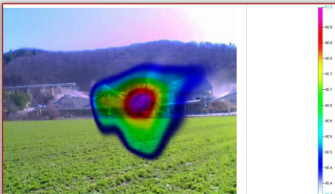
Figure 4. Noise visualization measurement of entire industrial area – south view
