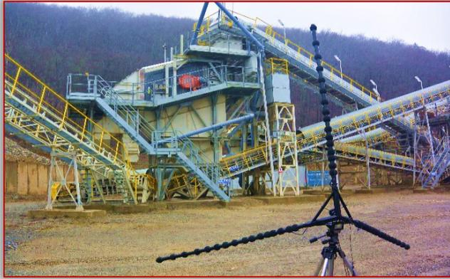
Figure 3. Installed acoustic camera
