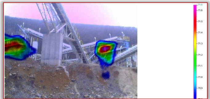
Figure 6. Noise visualization measurement of secondary line
