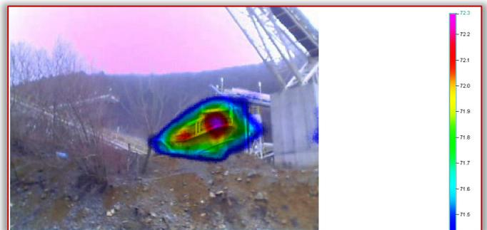
Figure 7. Noise visualization measurement of secondary line
