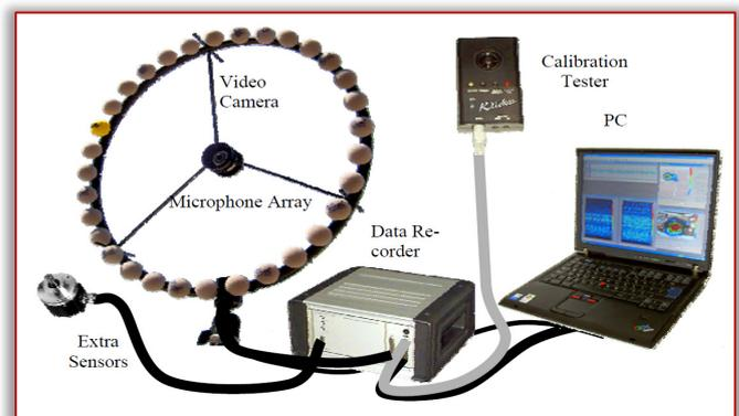
Figure 1. Basic component of noise visualization tools [11]
