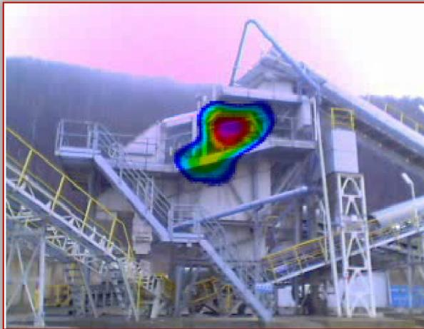
Figure 9. Noise visualization measurement of sorter 1
