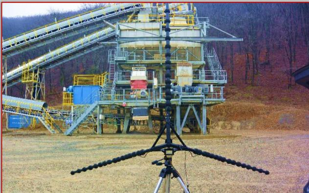
Figure 3. Installed acoustic camera
