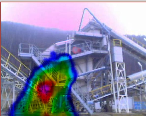
Figure 10. Noise visualization measurement of sorter 2
