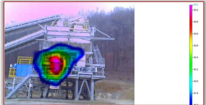
Figure 11. Noise visualization measurement of crusher
