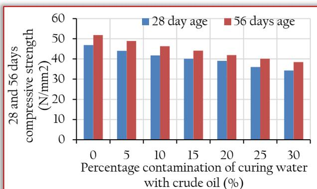
Figure 5. Relationship between the percentage contaminations of curing water with 28 and 56 days compressive strength of concrete specimens containing 20% sugar cane bagasse ash (SBA) and saw dust ash (SDA)
