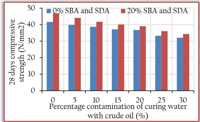
Figure 6. Relationship between the percentage contaminations of curing water with 28 days compressive strength of concrete specimens containing 0% and 20% sugar cane bagasse ash (SBA) and saw dust ash (SDA)
