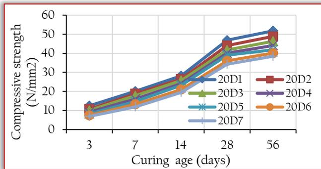
Figure 4. Relationship between the compressive strength and curing age of concrete specimens containing 20% sugar cane bagasse ash (SBA) and saw dust ash (SDA)
