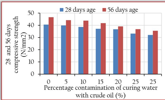
Figure 3. Relationship between the percentage contaminations of curing water with 28 and 56 days compressive strength of concrete specimens containing 0% sugar cane bagasse ash (SBA) and saw dust ash (SDA)
