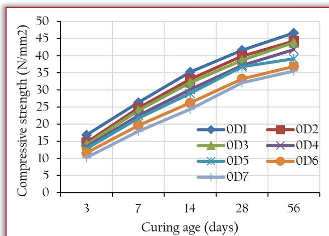
Figure 2. Relationship between the compressive strength and curing age of concrete specimens containing 0% sugar cane bagasse ash (SBA) and saw dust ash (SDA)
