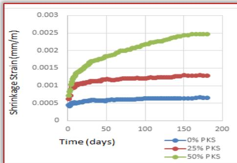
Figure 7: Drying shrinkage of palm kernel shell concrete
