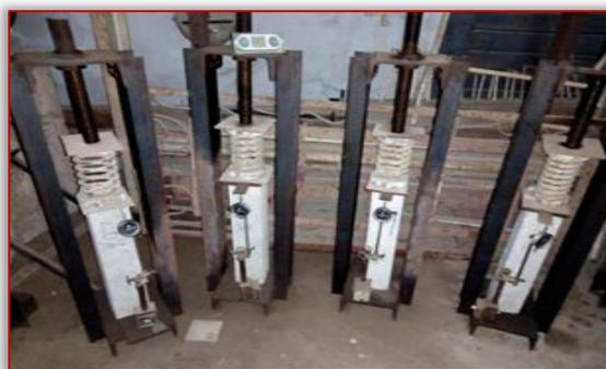
Figure 2: Specimens under creep test
