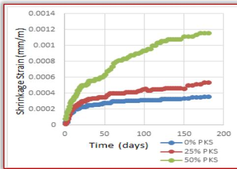
Figure 6: Basic shrinkage of palm kernel shell concrete
