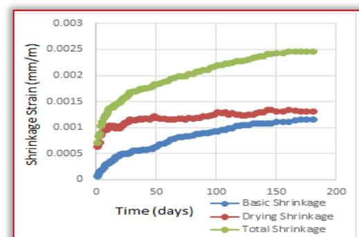
Figure 5: Shrinkage strain of 50% palm kernel shell concrete
