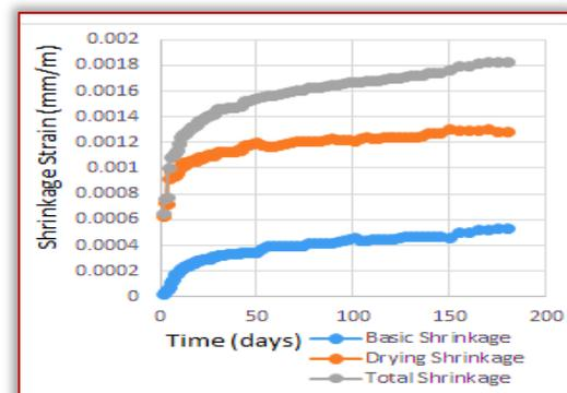
Figure 4: Shrinkage strain of 25% palm kernel shell concrete
