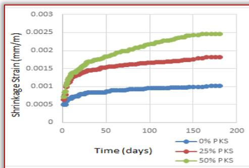
Figure 8: Total shrinkage of palm kernel shell concrete
