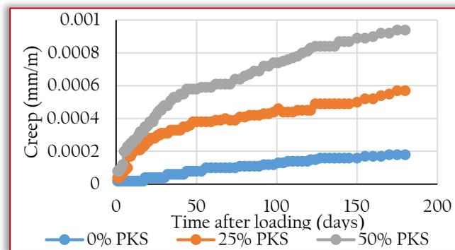
Figure 10: Creep of Palm Kernel Shell Concrete
