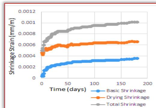
Figure 3: Shrinkage strain of normal concrete
