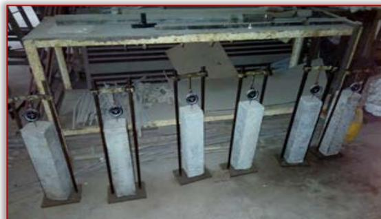
Figure 1: Specimens under shrinkage test
