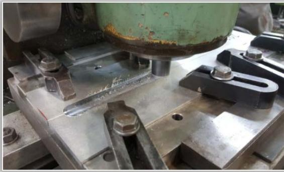
Figure 2. Machine for FSW welding
