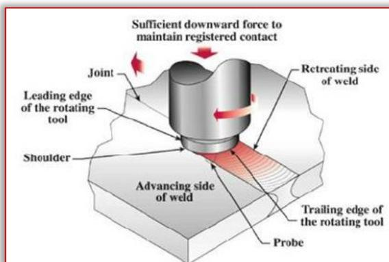
Figure 1. Illustrated scheme of friction stir welding
