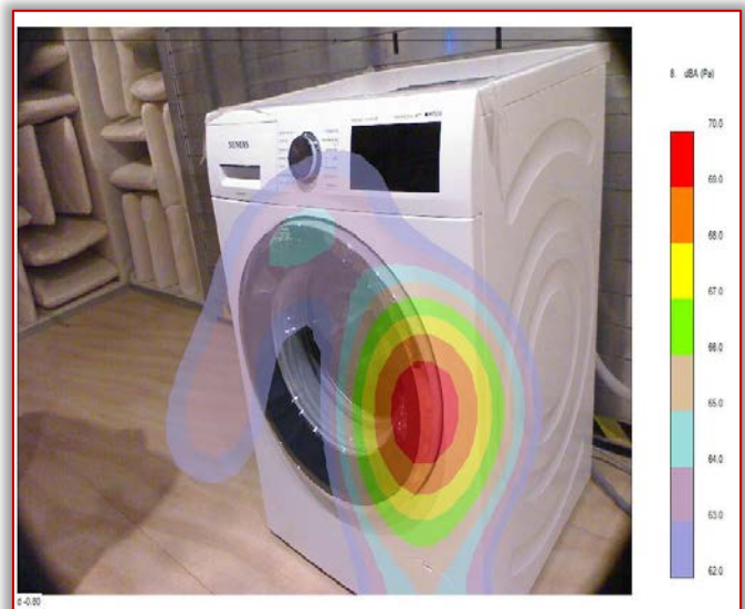
Figure 3. Visualization of sound from door closing, dominant frequencies 2300 – 2500 Hz
