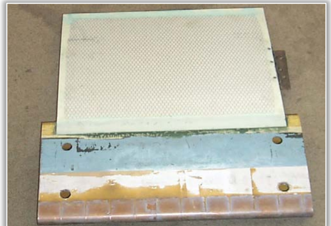
Figure 4. The composite segment with part spar
