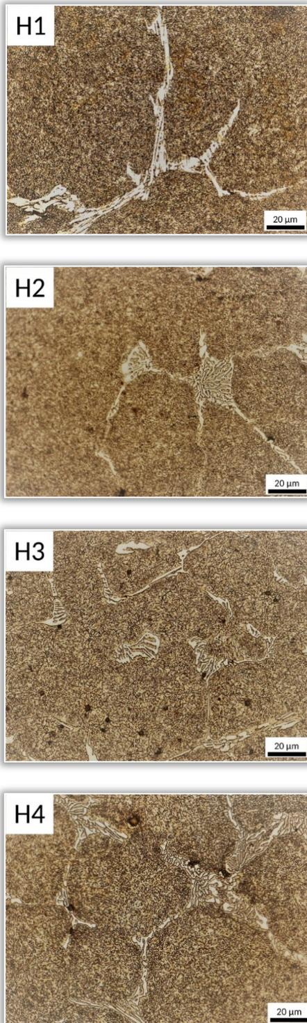
Figure 2. Optical Micrographs of Double Austenitization H1–H3
