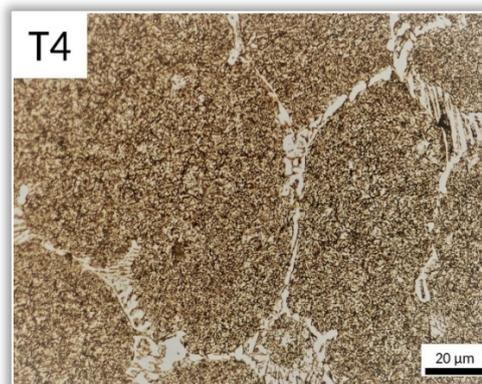
Figure 1. Optical Micrographs of Single Austenitisation T1–T4
