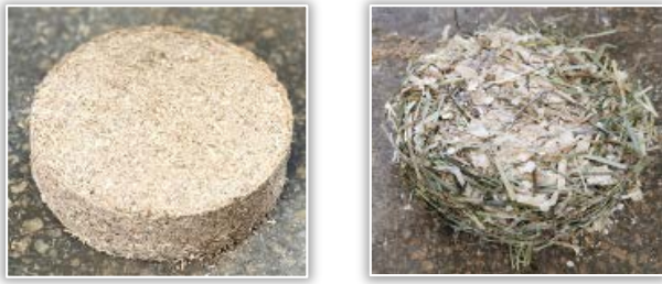
Figure 6 – Pellet samples obtained using the tableting equipment
