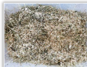
Figure 4 – Biomass mix used for obtaining tablets
