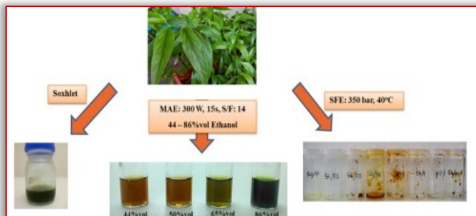
Figure 5. Extraction of phytochemicals from the medicinal plant Clinacanthus nutans Lindau by microwave-assisted extraction and supercritical carbon dioxide extraction (Popova A., 2018)
