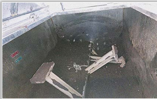
Figure 4. The operation of mixing and aerating the organic matter inside the equipment
