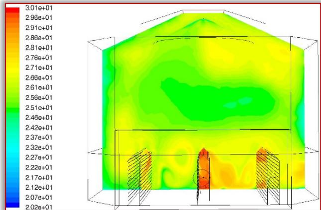
Figure 8 – Air temperature field in the transverse plane of the drying equipment (°C)
