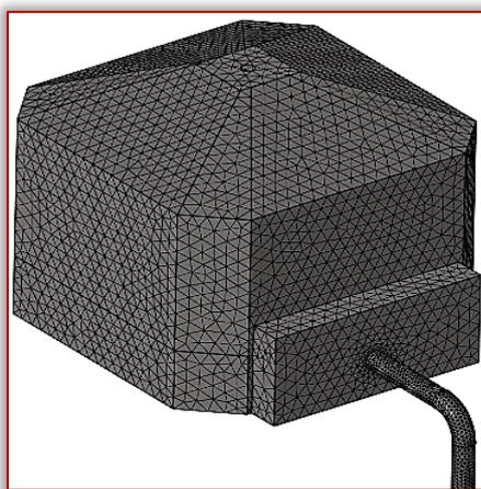
Figure 3 – Grid for geometry of the drying equipment
