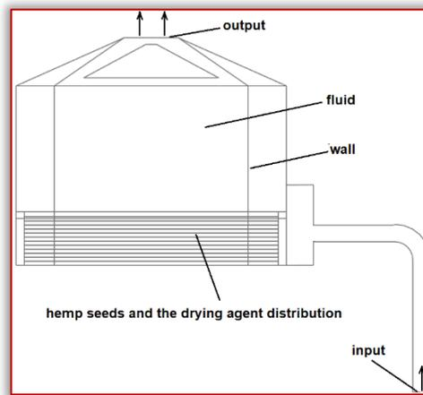
Figure 4 – Boundary condition for the CFD simulation
