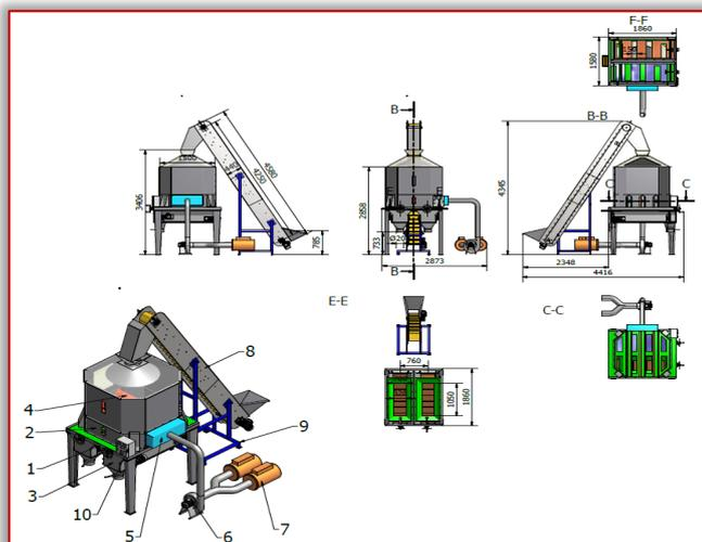
Figure 15 – Constructive diagram of the equipment
