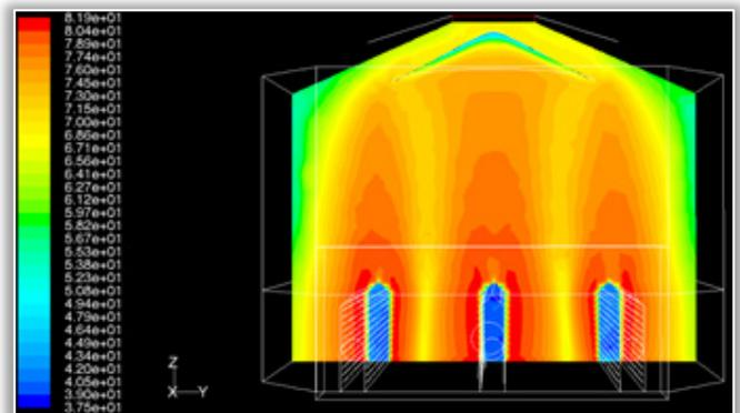
Figure 14 – The relative humidity of the warm air inside the drying equipment with hemp seeds in YOZ plane (%)
