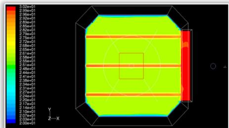
Figure 12 – Temperature field in the upper plane of the hemp seed layer (°C)
