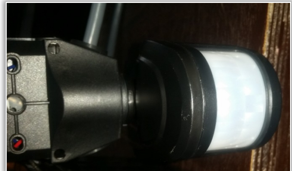
Figure 4: A Passive infrared (PIR) motion sensor used
