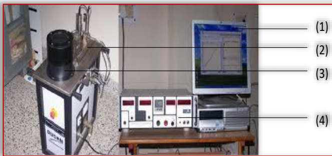
Figure 1: Pin-On-Disc Tribotester Set Up
