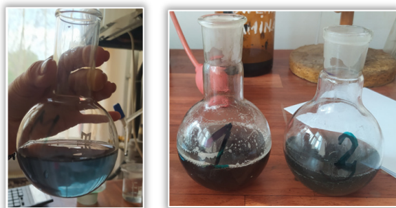
a) Figure 3. The control sample (a) and samples 1 & 2 (b) after titration with Mohr's salt
