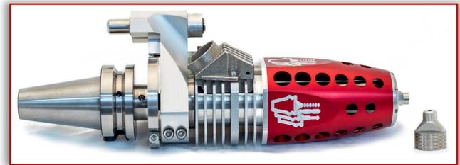
Figure 3. Laser DED extruder in a testing setup in a Haas VF series CNC machine [8]
