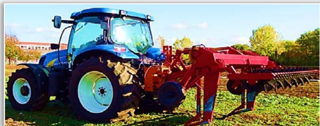
Figure 1. Technical equipment with active bodies trained for the work of loosening the soil in depth
