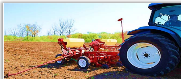
Figure 14. The technical equipment for tilling the soil in strips, sowing weeds, fertilizing and distributing insecticides
