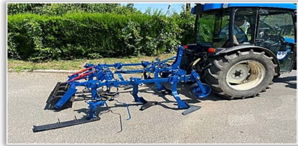
Figure 16. Weeding equipment for working in rows and between the vine trunks, EPV 2.2
