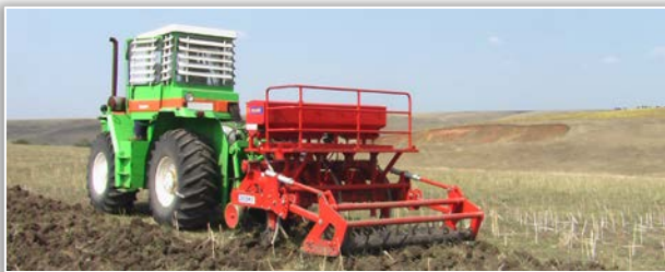
Figure 4. Decompactor for deficient soils with simultaneous administration of nutrients
