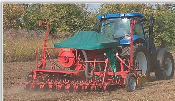
Figure 11. Technical equipment with working bodies for preparing the soil and sowing grassy cereals SGR
