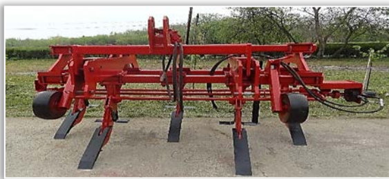
Figure 15. Equipment for working the soil in the substrate adapted to conservative technology
