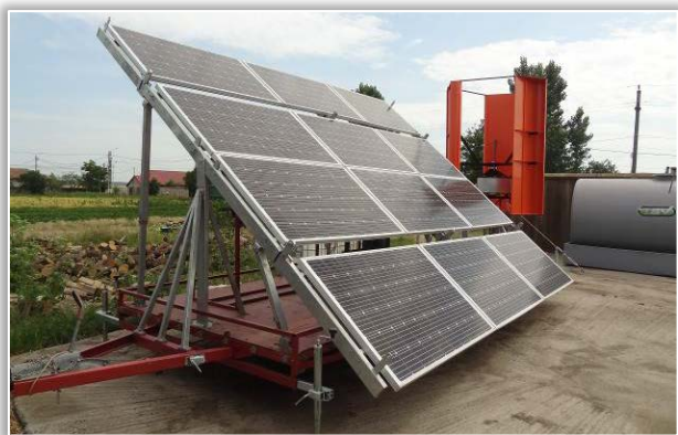
Figure 2. Trailer for transporting mobile electricity production system + photovoltaic installation
