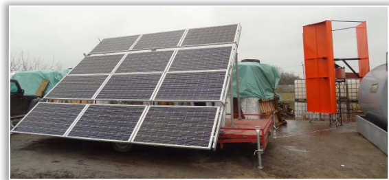
Figure 1. Mobile system for the production of electricity from alternative sources (solar + wind) for agricultural applications and monitoring, tele-transmission and crop management services
