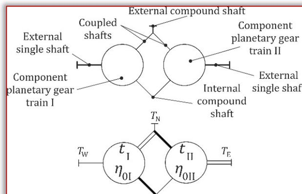
Figure 2. Two– carrier PGT symbol with shafts and respective torques marked. The torque markings of the external shaft torques ( $T_W$ ,  $T_N$  and  $T_E$ ) follow the cardinal directions (W, N, E), and are ordered from power input to power output. The symbol contains the markings of the ideal torque ratio ( $t_I$  and  $t_{II}$ ) and efficiency ( $\eta_{0I}$  and  $\eta_{0II}$ ) for every basic component PGT [10].
