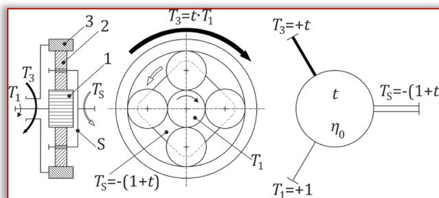
Figure 1. 1AI, the most used simple PGT with the specific torques on its shafts and its Wolf– Arnaudov symbol
