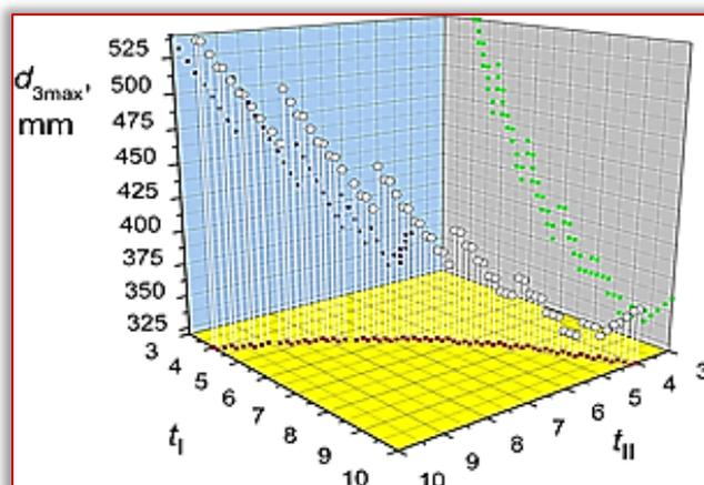
Figure 12. The influence of ideal torque ratios on maximal diameter of transmission in the example 2
