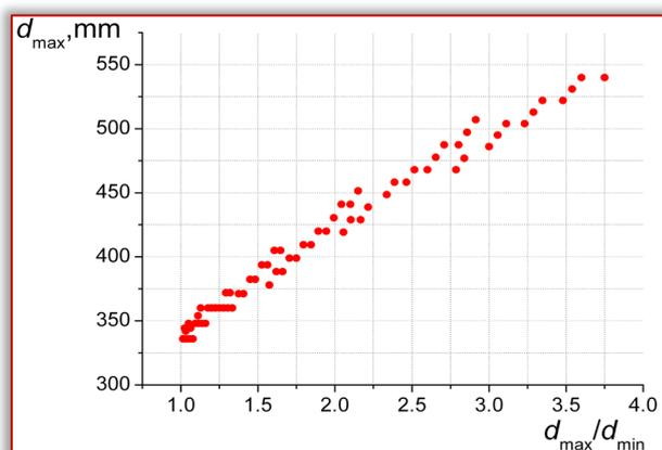
Figure 10. Correlation between maximal diameter of transmission and relation of ring gear reference diameters
