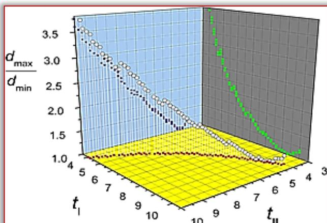
Figure 11. The influence of ideal torque ratios on the size ratio of the larger and smaller ring gears diameters
